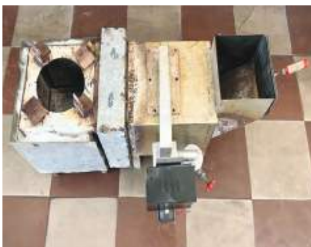
(d): Size: 3.5 kg/hr, Type: Horizontal, Forced draft cookstove
