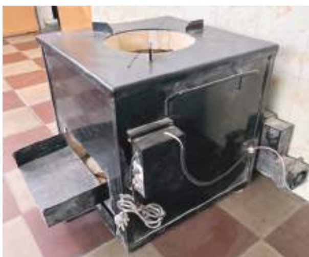
(c): Size: 15 kg/hr, Type: Vertical, Forced draft cookstove
