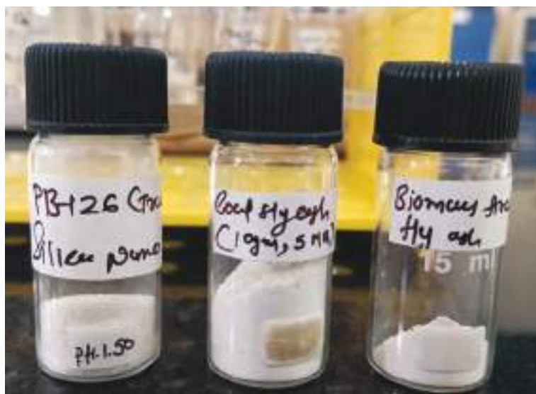
Extracted \text{SiO}_2 Nano particles from Rice straw (PB 126), Industrial coal fly ash, and Biomass fired fly ash with size ranging from 80-90 nm
