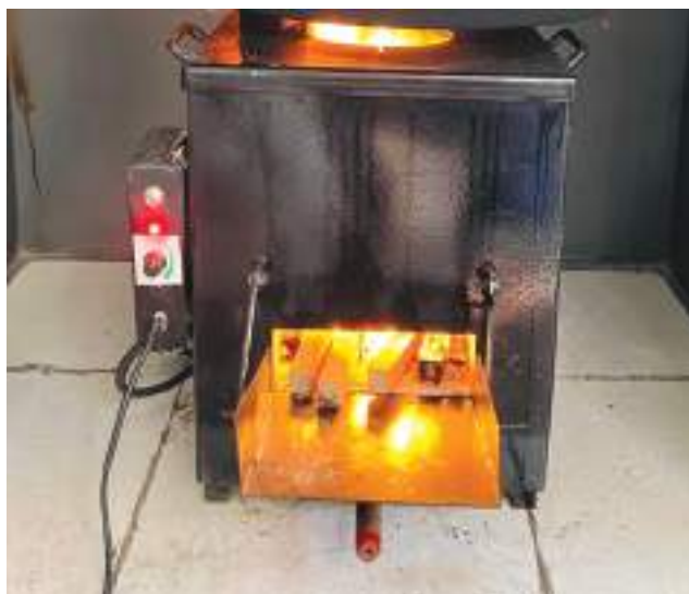
(b): Size: 3.5 kg/hr, Type: Vertical, Forced draft cookstove
