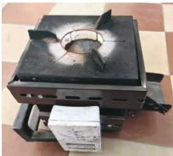
(a): Size: 1.5 kg/hr, Type: Vertical, Forced draft cookstove
