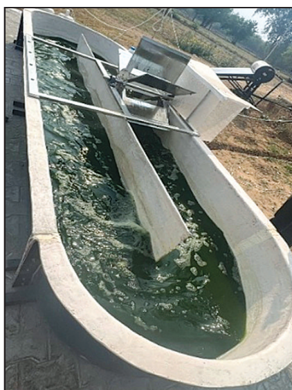
Algal biomass harvesting from the raceway pond and mixing of the harvested biomass
