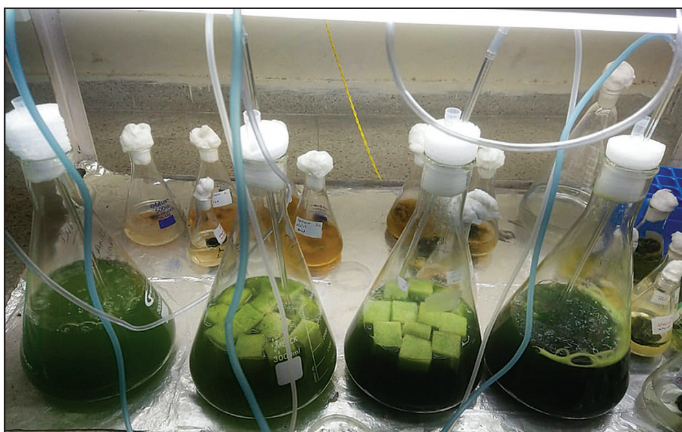
Biomass growth and attachment resulting in biofilm formation in the sponge media
