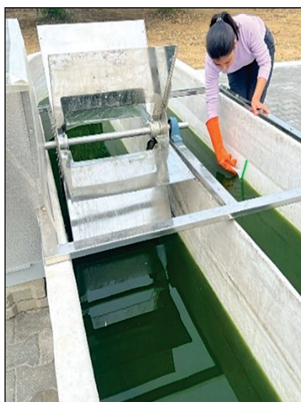
Algal biomass harvesting from the raceway pond and mixing of the harvested biomass
