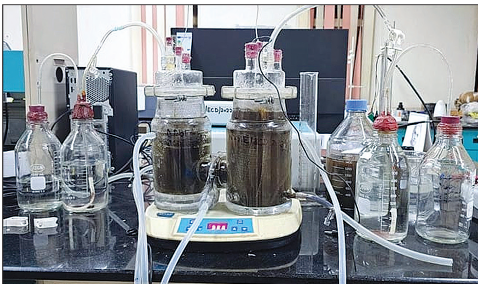
Reactor set-up for biogas upgradation via microbial electromethanogenesis
