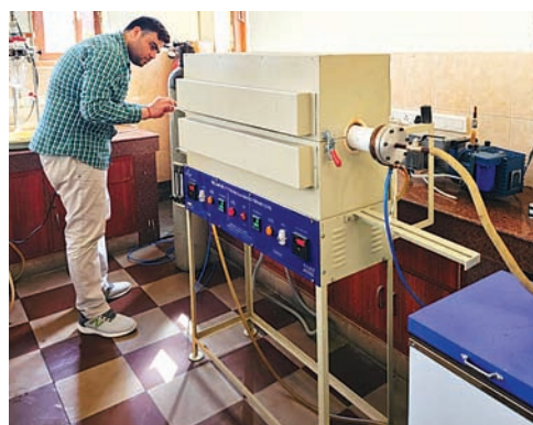
Synthesis of Biomass-derived carbon material through a two-zone tube furnace
