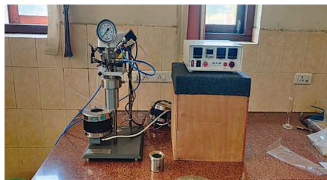
High pressure and temperature Reactor
