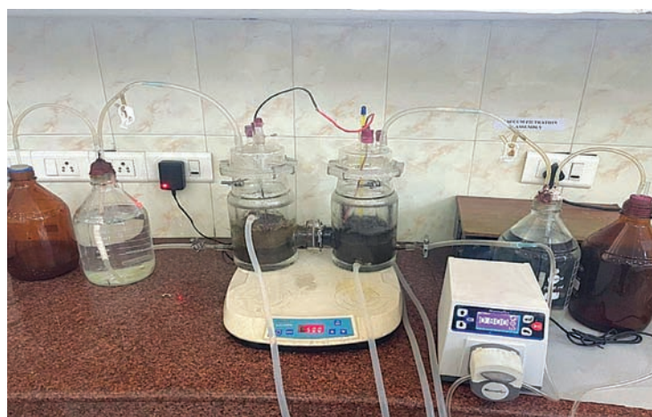
A jacketed double-chambered bioreactor (H-type cell) for the upgradation of biogas via microbial
